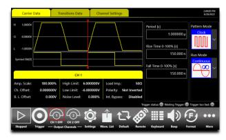
The software architecture provides the possibility to easily generate the patterns in different generation modality and also gives the opportunity to modulate the patterns with internal or external signals with the purpose to generate also different effects of noise (jitter, ripple, ...).
